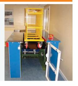
A lifting table designed and manufactured to be used as a work station.
